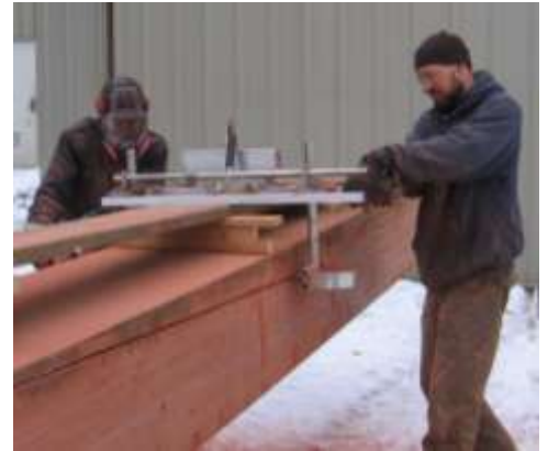
Dave Griswold and Chris Stohlman cutting the shape of the keel with a chainsaw mill
