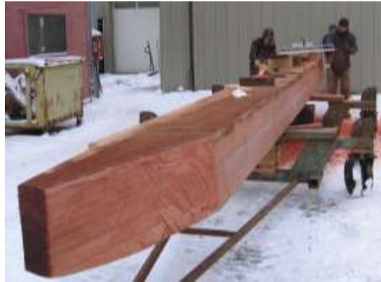
Dave Griswold and Chris Stohlman cutting the shape of the keel with a chainsaw mill
